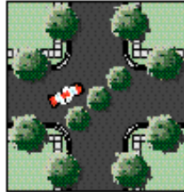
Diagonal Road Closure with Bollards
