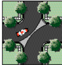
Diagonal Road Closure with Strip
